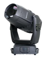
AQUA 480 Beam is a waterproof and IP66 rated fixture. It has beam angle of 2° with sharp edges. It can produce a number of effects via CMY system, 18 fixed gobos ,7 rotating gobos and etc.. It is ideal for outdoor entertainment, concerts and etc..
